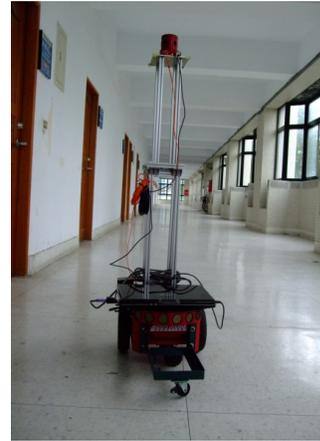
Figure 2. The mobile robot with a spherical camera with 1.6 meters height.
